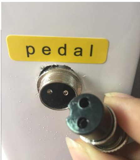
9. Plug the foot switch and remote switch
