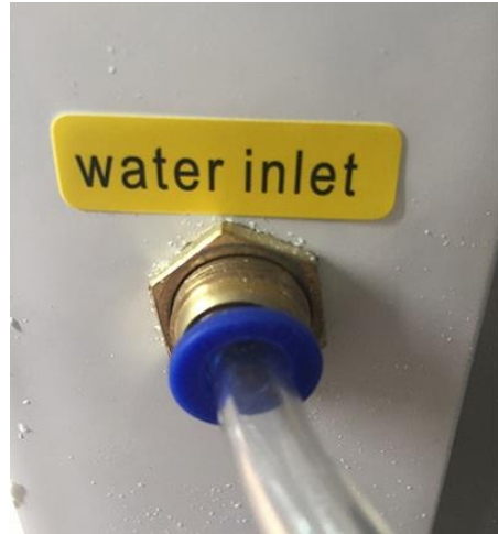
6. Connected the filling funnel and tighten it, add water until the water overfall come out of water, then it's completed
