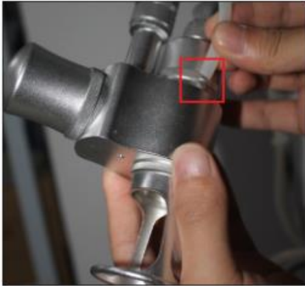
5. Connect the gas-guide tube on the graphics generator
